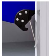
In case of a collision, the closing edge can bend in all directions. Pre-stressed ropes ensure a controlled deformation until the snap-in connections between the edge of the door leaf and the guide pieces disconnect. Subsequently, the door curtain can slip out of the door frame guides in any direction.
