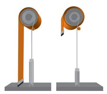
Tension springs are installed in the side frames and directly connected to the drive shaft by heavy load belts. The springs are taut in the position "Door is closed" (left) and slack in the position "Door is open".
